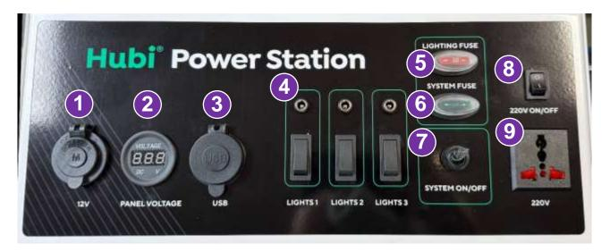
To turn the system on, click the system on/off switch (7) into the forward position. The panel voltage display (2) will come on and indicate the current battery voltage.
